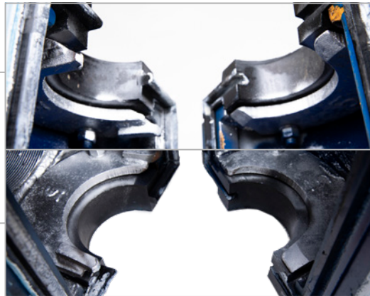
METAL END SEAL BUMPER PLATES PROTECT THE SEAL
